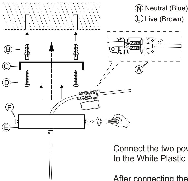
Connect the two power wires coming out from the ceiling to the White Plastic Connector (A).
