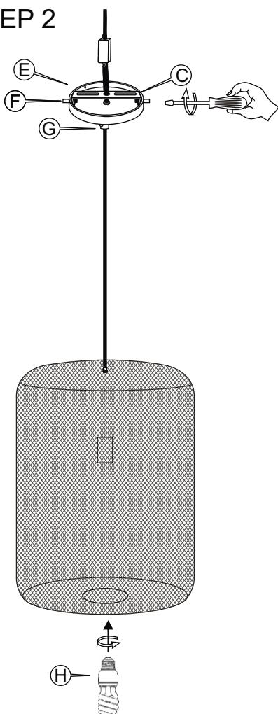
Tighten the canopy (E) with side Screw (F) to the mounting plate (C) and tighten the screw on plastic cord grip (G)
